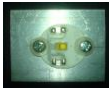
Use metal screw with nylon washer
